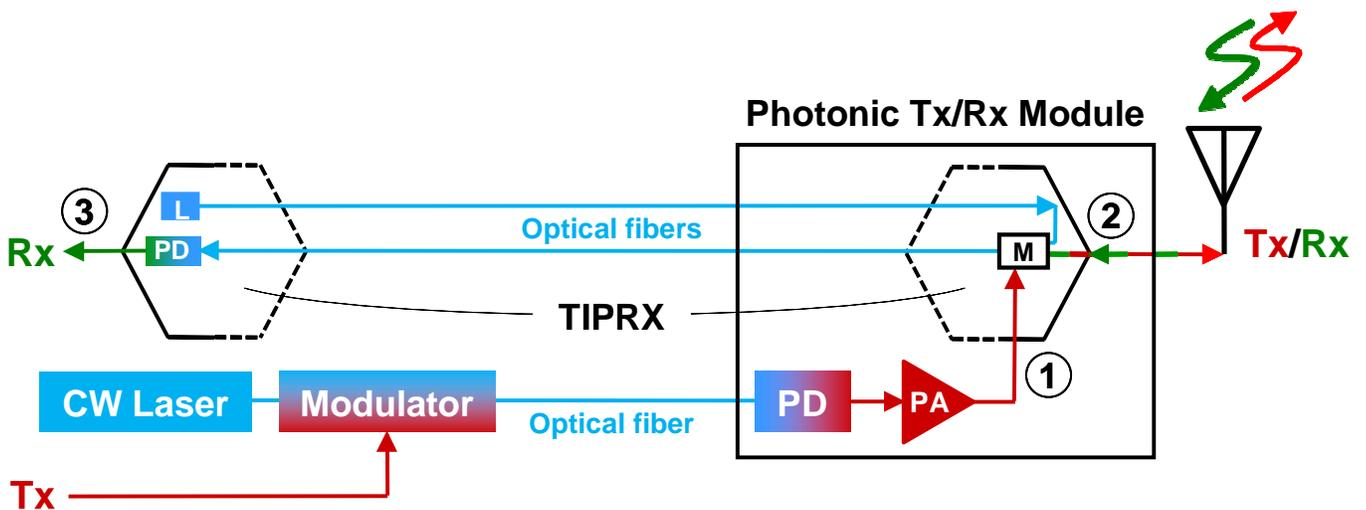
Fig. 3 Splitting apart of the TIPRX into the modulator portion at the antenna site and the CW laser and high-speed photodetector for the receive signal, both of which can be located at a remote site along with the Tx signal generator and the receiver for the Rx signal.
