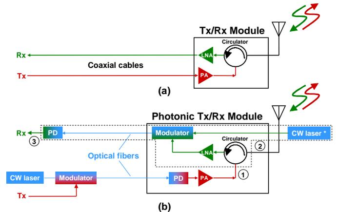
Fig. 1 (a) Conventional Tx/Rx antenna interface module. PA: power amplifier. (b) Addition of photonic components to the conventional module to enable remoting of the Tx and Rx signals via optical fibers. The dashed box and port numbers are explained in Section II. \*CW laser power can be delivered to the module via a third optical fiber.
