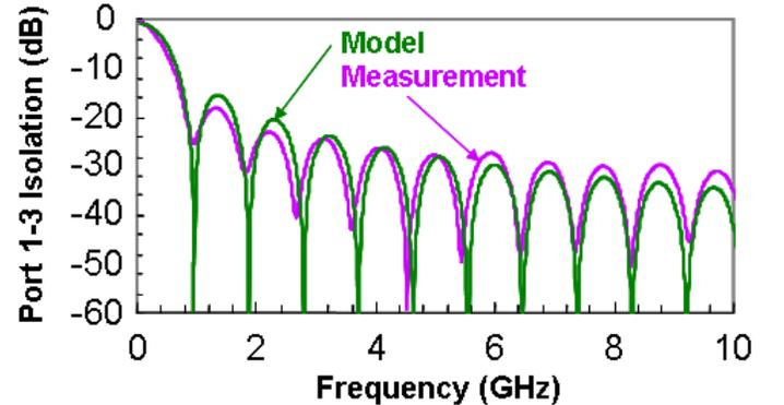
Fig. 4 Measured port 1 – 3 isolation of a TIPRX (magenta curve) with RF reflections “gated” out of the network analyzer measurements of  $S_{31}$  and  $S_{32}$  in an early experiment to validate the simple model (green curve) expressed in (1) and (2).
