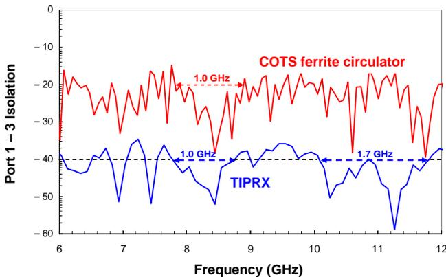
Fig. 5 Measured port 1 – 3 isolation of a TIPRX designed to minimize the deleterious effects of RF reflections at 6 – 12 GHz (blue curve). Better than –35 dB of port 1 – 3 isolation was achieved across the entire octave, and better than –40 dB of port 1 – 3 isolation was achieved across two bands of width 1.0 GHz and 1.7 GHz. The measured isolation for the best 6 – 12 GHz commercial ferrite-based RF circulator [7] is shown for comparison (red curve).
