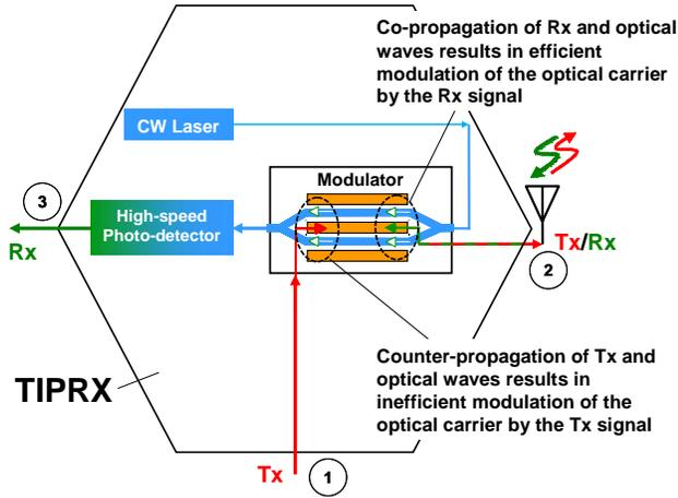
Fig. 2 Block diagram of the Transmit-Isolating Photonic Rx link (TIPRX). The three components inside the hexagon replace the five components inside the irregularly shaped dashed box shown in Fig. 1(b), with corresponding numbering of the three RF signal ports.
