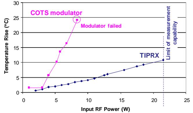
Fig. 6 Results of step stress tests, showing the TIPRX’s improved RF power handling capability compared to that of a COTS modulator.
