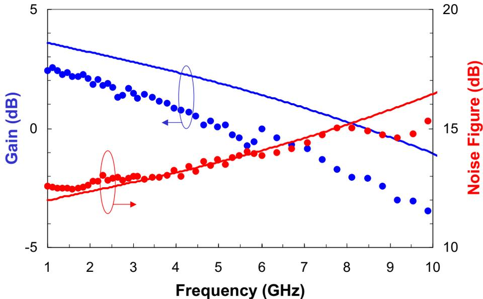
**Fig. 3** Measured (points) and modeled (lines) link Gain and Noise Figure for the link diagrammed in Fig. 2. Parameters used in the model are listed in Section IV.
