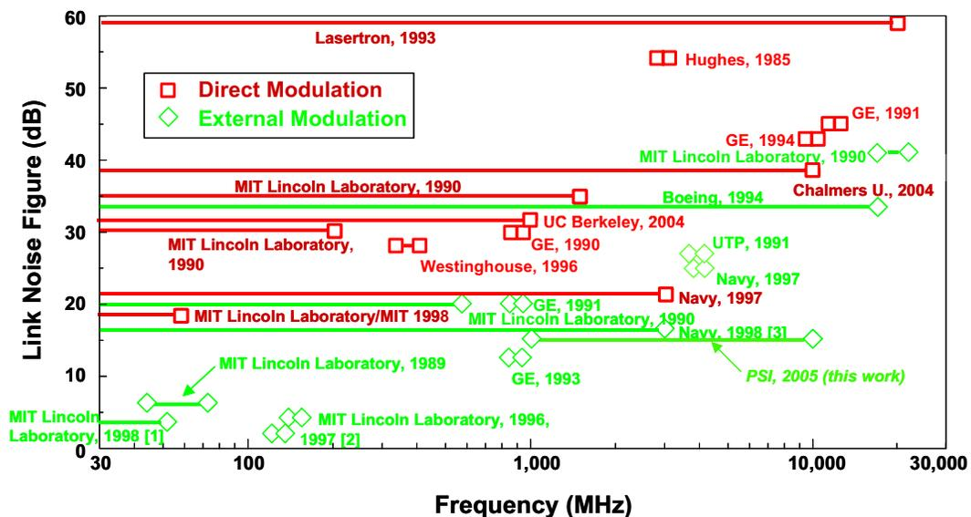
Fig. 1 Measured noise figures of intrinsic direct and external modulation analog optical links.
