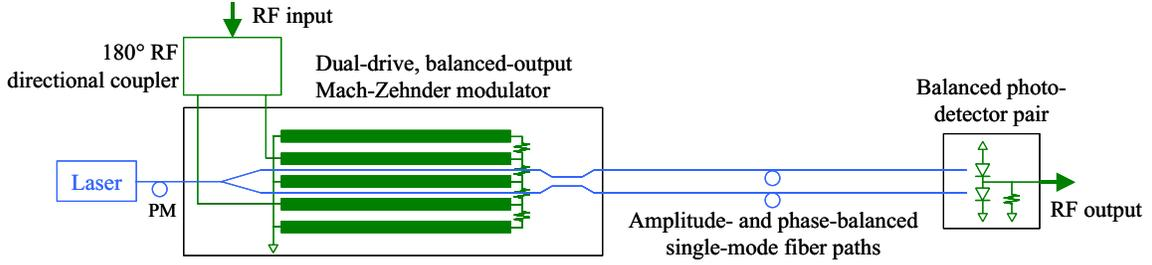
**Fig. 2** Block diagram experimental analog optical link with low intrinsic noise figure.
