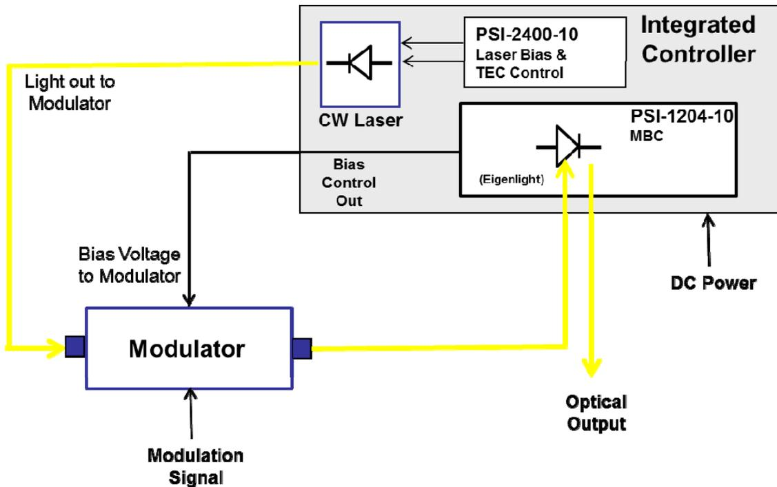
The PSI-2400-10 LDC and PSI-1204-10 have been designed and tested to operate over a wide operating temperature range of -40 to +85°C.
