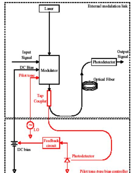
MBC does not include a feedback photodetector or tap coupler. For the majority of applications, a photodetector such as Fermionics model FD-300 or equivalent is suggested. The tap coupler should be selected based on the optical power present at the output of the modulator does not exceed 320uA at Max, or equal to 160 uA at Quad.
