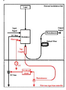
MBC does not include a feedback photodetector or tap coupler. For the majority of applications, a photodetector such as Fermionics model FD-300 or equivalent is suggested. The tap coupler should be selected based on the optical power present at the output of the modulator does not exceed 320uA at Max, or equal to 160 uA at Quad.
